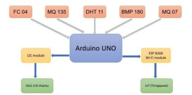
The I2C module allows multiple devices to be connected to each other using just two wires. The screen will show on the 16\*2 LCD. In addition, the ESP8266 Wi-fi module is used to enable ,internet connectivity with various vehicle system applications and will provide data for subsequent jobs i.e. the website will also show the output to the user on the screen with the data graph and also store it in the database.
