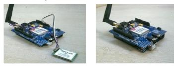
Figure 5. GPS module with Arduino board Figure 6. GSM module with Arduino
