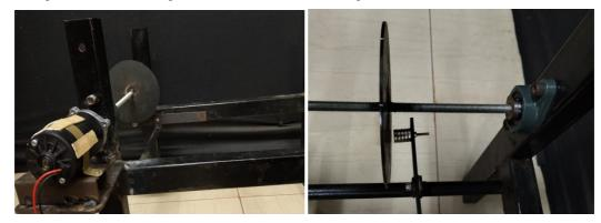
Fig. 8 Realized working model of preliminary Braking system using PMs Fig. 9. View of PMs in vicinity of the Brake disc
